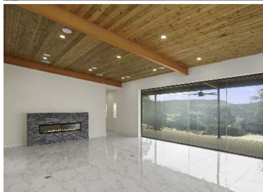
FRAMELESS WINDOW WALL — LAMINATED GLASS
